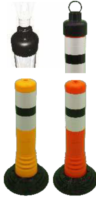
12234 KG PingPong™ Post yellow 12236 KO PingPong™ Post orange (H)450 mm, TPU, ø 80 mm, 1,10 kg reflective tapes ORALITE® 5450 white Commercial Grade Class RA1 Design A Foot ABS ø 200 mm for conglunation 41,95 €/pc.
