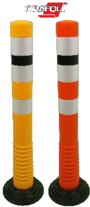
12230 KG PingPong™ Post yellow 12232 KO PingPong™ Post orange (H)750 mm, TPU, ø 80 mm, 1,46 kg reflective tapes ORALITE® 5450 Commercial Grade Class RA1 Design A Foot ABS ø 200 mm for conglunation 49,95 €/pc.
